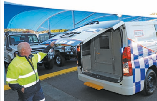
Wayne Denman from Fleet Assets demonstrates the tailgate lift and cargo floor height for pod entry.
