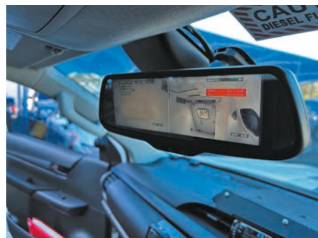
The pod surveillance camera is linked to the vehicles rear view mirror.
