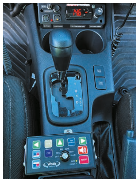
The New Zealand made WADE siren/light system control panel that has flexible options for officers to utilise the warning devices.
