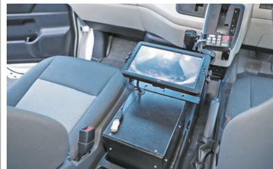
The surveillance camera screen and download connection cables. The system can be replayed direct from the screen to check on the prisoners welfare.
