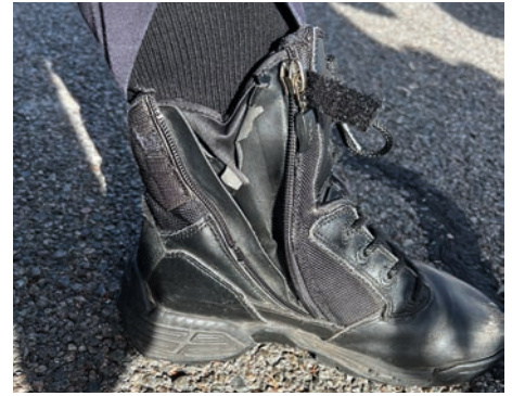
Broken zips, velcro strips tearing off and soles delaminating are common complaints about the current models that are being issued to frontline officers.
